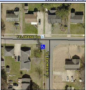
**FELDBANK DR** Street 1 Name Stop Condition-Street 1 None N/A Street 2 Name Stop Condition-Street 2 N/A Possible Solutions: Compliance Description Remove & Replace Curb Ramp With Two New Directional Ramps or Equivalent. Surveyor Notes: N/A PROW/ADA: Not Found, R304.5.1
