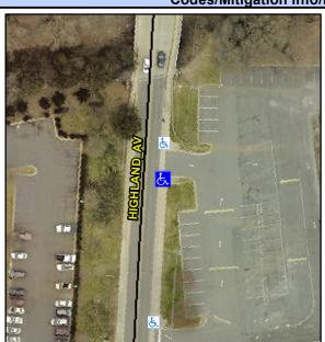
**ENTRANCE** Street 1 Name Stop Condition-Street 2 None Street 2 Name **HIGHLAND AV** Stop Condition-Street 1 None Possible Solutions: Remove & Replace Curb Ramp With **Two New Directional Ramps or** Equivalent. Surveyor Notes: N/A PROW/ADA: R304.5.3
