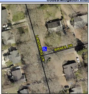
Street 1 Name Stop Condition-Street 2 Street 2 Name Stop Condition-Street 1 LANDSBURG LN None **BIRNEN DR** StopSign Remove & Replace Curb Ramp With Two New Directional Ramps or Equivalent.
