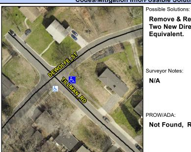
**TILLMAN RD** Street 1 Name Stop Condition-Street 1 StopSign Street 2 Name N/A Stop Condition-Street 2 N/A Remove & Replace Curb Ramp With **Two New Directional Ramps or** Equivalent.
