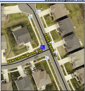
ARMSTRONG PARK DR Street 1 Name Stop Condition-Street 2 StopSign **BASIE PARK CT** Street 2 Name Stop Condition-Street 1 None Possible Solutions: Compliance Description N/A Remove & Replace Curb Ramp With Two New Directional Ramps or Equivalent. Surveyor Notes: N/A PROW/ADA: Not Found, R304.5.1, R304.5.3
