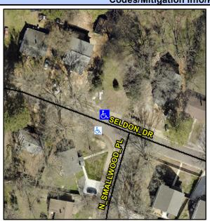
**SELDON DR** Street 1 Name Stop Condition-Street 1 None Street 2 Name N/A Stop Condition-Street 2 N/A Possible Solutions: Remove & Replace Curb Ramp With Two New Directional Ramps or Equivalent. Surveyor Notes: **VEGETATION OVERGROWTH** PROW/ADA: Not Found, R304.5.3
