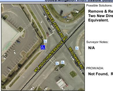
MT HOLLY HUNTERSVILLE RD Street 1 Name Stop Condition-Street 1 Signal Street 2 Name N/A Stop Condition-Street 2 N/A Remove & Replace Curb Ramp With **Two New Directional Ramps or** Equivalent.
