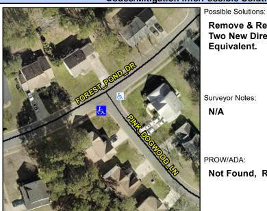
**PINK DOGWOOD LN** Street 1 Name Stop Condition-Street 1 StopSign Street 2 Name N/A Stop Condition-Street 2 N/A Remove & Replace Curb Ramp With Two New Directional Ramps or Equivalent.
