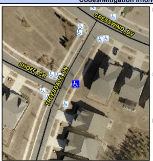
TREESDALE LN Street 1 Name Stop Condition-Street 2 None Street 2 Name N/A Stop Condition-Street 1 N/A Possible Solutions: Remove & Replace Entire Ramp. Grind Gutter Lip. Surveyor Notes: N/A PROW/ADA: R304.5.3, R305.2, R302.7.2
