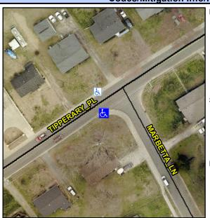
**TIPPERARY PL** Street 1 Name Stop Condition-Street 1 None Street 2 Name N/A Stop Condition-Street 2 N/A Possible Solutions: Remove & Replace Entire Ramp. Surveyor Notes: RT RP < 5% PROW/ADA: R304.3.2, R304.5.3
