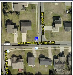
NORTHWOODS FOREST DR Street 1 Name Stop Condition-Street 1 None N/A Street 2 Name Stop Condition-Street 2 N/A Possible Solutions: Remove & Replace Curb Ramp With Two New Directional Ramps or Equivalent. Surveyor Notes: N/A PROW/ADA: Not Found, R304.5.1, R304.5.3
