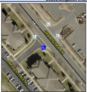
**GRANDIFLORA DR** Street 1 Name Stop Condition-Street 2 None **ENTRANCE** Street 2 Name Stop Condition-Street 1 StopSign Possible Solutions: Remove & Replace Curb Ramp With Two New Directional Ramps or Equivalent. Surveyor Notes: N/A PROW/ADA: R304.5.1, R304.2.2
