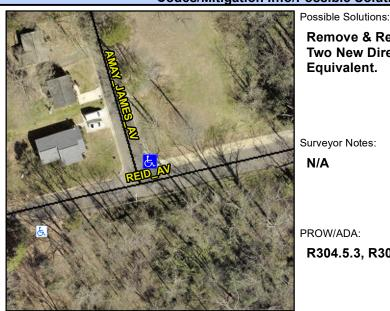
Street 1 Name StopSign Stop Condition-Street 1 **AMAY JAMES AV** Street 2 Name None Stop Condition-Street 2 **REID AV**  Remove & Replace Curb Ramp With Two New Directional Ramps or Equivalent.
