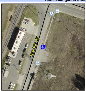
**TEXLAND BV** Street 1 Name Stop Condition-Street 2 None Street 2 Name **ENTRANCE** Stop Condition-Street 1 None Possible Solutions: Remove & Replace Curb Ramp With **Two New Directional Ramps or** Equivalent. Surveyor Notes: N/A PROW/ADA: Not Found, R304.2.2
