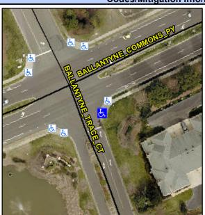
**BALLANTYNE TRACE CT** Street 1 Name Stop Condition-Street 2 StopSign Street 2 Name N/A Stop Condition-Street 1 N/A Possible Solutions: Remove & Replace Entire Ramp. Surveyor Notes: N/A PROW/ADA: Not Found, R304.5.1, R304.2.2, R304.5.3
