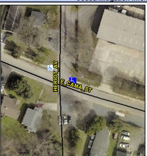
**HERIOT AV** Street 1 Name Stop Condition-Street 2 None Street 2 Name **E CAMA ST** Stop Condition-Street 1 None Possible Solutions: Remove & Replace Curb Ramp With **Two New Directional Ramps or** Equivalent. Surveyor Notes: N/A PROW/ADA: Not Found, R304.2.2, R304.5.3
