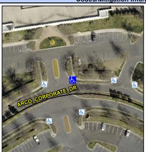
**ENTRANCE** Street 1 Name Stop Condition-Street 2 None ARCO CORPORATE DR Street 2 Name Stop Condition-Street 1 None Possible Solutions: Remove & Replace Curb Ramp With Two New Directional Ramps or Equivalent. Surveyor Notes: N/A PROW/ADA: Not Found, R304.5.1
