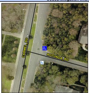
**ROTUNDA RD** Street 1 Name Stop Condition-Street 2 StopSign Street 2 Name N/A Stop Condition-Street 1 N/A Possible Solutions: Remove & Replace Entire Ramp. Surveyor Notes: N/A PROW/ADA: R304.5.1, R304.2.2
