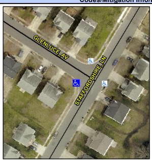
STAFFORDSHIRE LN Street 1 Name Stop Condition-Street 2 None **GLENLUCE AV** Street 2 Name Stop Condition-Street 1 StopSign Possible Solutions: Remove & Replace Curb Ramp With Two New Directional Ramps or Equivalent. Surveyor Notes: N/A PROW/ADA:
