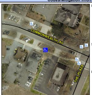
**COMMONWEALTH AV** Street 1 Name Stop Condition-Street 2 None Street 2 Name N/A Stop Condition-Street 1 N/A Possible Solutions: Remove & Replace Entire Ramp. Surveyor Notes: N/A PROW/ADA: R304.5.3, R304.2.3, R305.2
