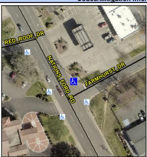
Street 1 Name Stop Condition-Street 2 Street 2 Name Stop Condition-Street 1 **NATIONS FORD RD** None **FARMHURST DR** StopSign Possible Solutions: Remove & Replace Curb Ramp With Two New Directional Ramps or Equivalent. Surveyor Notes: N/A PROW/ADA: Not Found, R304.2.2
