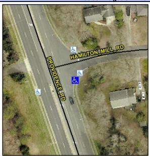
**PROVIDENCE RD** Street 1 Name Stop Condition-Street 2 None Street 2 Name N/A Stop Condition-Street 1 N/A Possible Solutions: Remove & Replace Entire Ramp. Surveyor Notes: N/A PROW/ADA: Not Found, R304.5.1, R304.2.2
