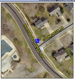
**COLIN CREEK LN** Street 1 Name StopSign Stop Condition-Street 1 Street 2 Name N/A Stop Condition-Street 2 N/A Possible Solutions: Remove & Replace Curb Ramp With **Two New Directional Ramps or** Equivalent. Surveyor Notes: N/A PROW/ADA:
