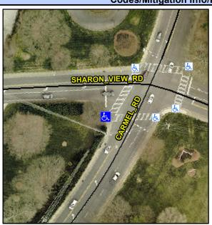
**CARMEL RD** Street 1 Name Stop Condition-Street 2 Signal **SHARON VIEW RD** Street 2 Name Stop Condition-Street 1 Signal Possible Solutions: N/A Remove & Replace Curb Ramp With Two New Directional Ramps or No Equivalent. Surveyor Notes: N/A PROW/ADA: Not Found, R304.5.1
