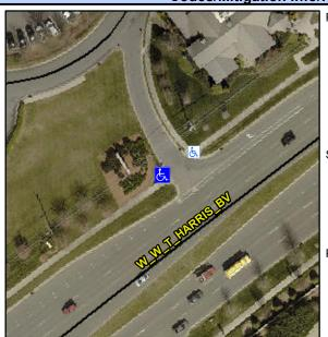
Street 1 Name **ENTRANCE** Stop Condition-Street 2 None Street 2 Name N/A Stop Condition-Street 1 N/A Possible Solutions: Remove & Replace Entire Ramp. Grind Gutter Lip. Surveyor Notes: N/A PROW/ADA: R304.5.3, R304.2.1, R304.2.2-Perp, R304.3.2-Para, R302.7.2
