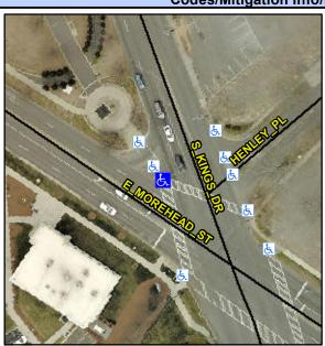
Street 1 Name Stop Condition-Street 2 Street 2 Name Stop Condition-Street 1 **PROVIDENCE RD** Signal **S KINGS DR** Signal Possible Solutions: Remove & Replace Curb Ramp With **Two New Directional Ramps or** Equivalent. Surveyor Notes: N/A PROW/ADA: Not Found, R304.5.3
