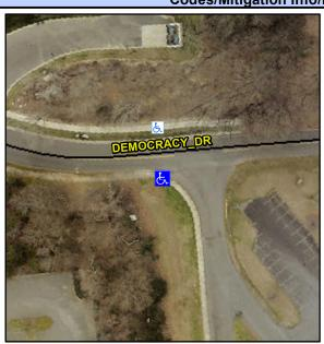
**ENTRANCE** Street 1 Name Stop Condition-Street 2 StopSign **DEMOCRACY DR** Street 2 Name Stop Condition-Street 1 None Possible Solutions: Remove & Replace Curb Ramp With **Two New Directional Ramps or** Equivalent. Surveyor Notes: N/A PROW/ADA: R304.5.1, R304.2.2, R304.5.3
