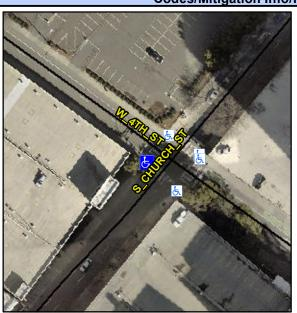
S CHURCH ST Street 1 Name Stop Condition-Street 2 Signal W 4TH ST Street 2 Name Stop Condition-Street 1 Signal Possible Solutions: Remove & Replace Curb Ramp With Two New Directional Ramps or Equivalent. Surveyor Notes: N/A PROW/ADA: Not Found, R304.5.1, R304.5.3
