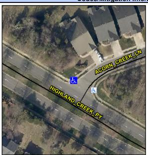
**ACORN CREEK LN** Street 1 Name Stop Condition-Street 2 StopSign Street 2 Name N/A Stop Condition-Street 1 N/A Possible Solutions: Remove & Replace Entire Ramp. Surveyor Notes: N/A PROW/ADA: R304.2.2, R304.5.3
