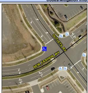
Street 1 Name Stop Condition-Street 2 Street 2 Name Stop Condition-Street 1 **NEW FASHION WY** None **OUTLETS BV** StopSign Possible Solutions: Remove & Replace Curb Ramp With Two New Directional Ramps or Equivalent. Surveyor Notes: N/A PROW/ADA: R304.5.3
