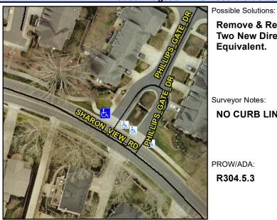
**PHILLIPS GATE DR** Street 1 Name Stop Condition-Street 1 StopSign Street 2 Name N/A Stop Condition-Street 2 N/A **Remove & Replace Curb Ramp With** Two New Directional Ramps or Equivalent.
