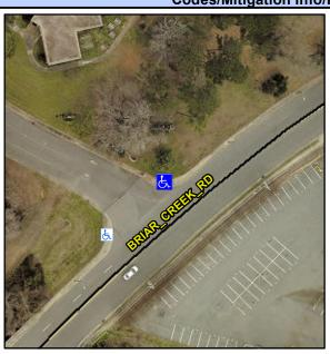
Street 1 Name Stop Condition-Street 1 Street 2 Name Stop Condition-Street 2 **BRIAR CREEK RD**  Possible Solutions: Remove & Replace Curb Ramp With Two New Directional Ramps or Equivalent. Surveyor Notes: **PONDING ON RAMP, LT RP < 5%** PROW/ADA: Not Found, R304.5.1, R304.5.1, R304.5.3, R304.3.2
