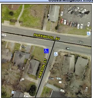
**PARSON ST** Street 1 Name Stop Condition-Street 1 StopSign N/A Street 2 Name Stop Condition-Street 2 N/A Possible Solutions: Remove & Replace Curb Ramp With Two New Directional Ramps or Equivalent. Remove & Replace Gutter.
