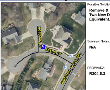
**KEELS CT** None N/A Possible Solutions: Remove & Replace Curb Ramp With Two New Directional Ramps or Equivalent.
