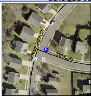
**JORDANS POND LN** Street 1 Name Stop Condition-Street 2 None Street 2 Name **SENEY DR** Stop Condition-Street 1 StopSign Possible Solutions: Remove & Replace Curb Ramp With **Two New Directional Ramps or** Equivalent. Surveyor Notes: N/A PROW/ADA: Not Found, R304.5.3
