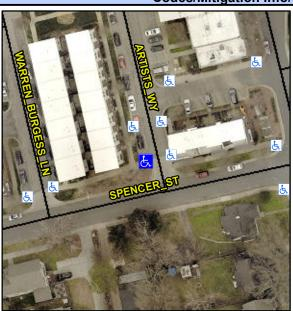
**ARTISTS WY** Street 1 Name Stop Condition-Street 1 StopSign Street 2 Name N/A Stop Condition-Street 2 N/A Possible Solutions: Remove & Replace Curb Ramp With **Two New Directional Ramps or** Equivalent. Surveyor Notes: **COLLECTED WITH ULIP**
