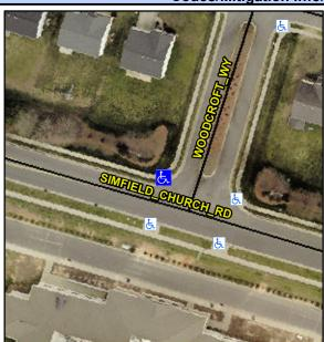
SIMFIELD CHURCH RD Street 1 Name Stop Condition-Street 2 None **WOODCROFT WY** Street 2 Name Stop Condition-Street 1 StopSign Possible Solutions: Remove & Replace Curb Ramp With Two New Directional Ramps or Equivalent. Surveyor Notes: N/A PROW/ADA: R304.5.3
