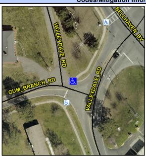
**VALLEYDALE RD** Street 1 Name StopSign Stop Condition-Street 1 Street 2 Name N/A Stop Condition-Street 2 N/A Remove & Replace Curb Ramp With **Two New Directional Ramps or** Equivalent.
