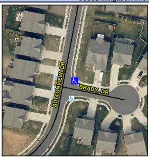
Street 1 Name Stop Condition-Street 2 Street 2 Name Stop Condition-Street 1 SUTTONVIEW DR None **BRADY DR** StopSign Possible Solutions: Remove & Replace Curb Ramp With Two New Directional Ramps or Equivalent. Surveyor Notes: N/A PROW/ADA: Not Found, R304.5.1, R304.5.3
