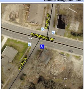
**ALLEN ST** Street 1 Name Stop Condition-Street 1 StopSign N/A Street 2 Name Stop Condition-Street 2 N/A Possible Solutions: Remove & Replace Curb Ramp With Two New Directional Ramps or Equivalent. Surveyor Notes:
