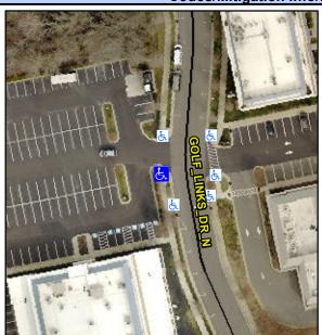
Street 1 Name **GOLF LINKS DR N** Stop Condition-Street 2 StopSign **ENTRANCE** Street 2 Name Stop Condition-Street 1 StopSign Possible Solutions: Remove & Replace Curb Ramp With Two New Directional Ramps or Equivalent. Surveyor Notes: N/A PROW/ADA: Not Found, R304.2.2
