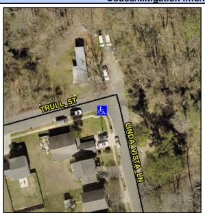
**LINDA VISTA LN** Street 1 Name Stop Condition-Street 1 **TRULL ST** Street 2 Name Stop Condition-Street 2 StopSign Possible Solutions: Remove & Replace Curb Ramp With Two New Directional Ramps or Equivalent. Surveyor Notes: N/A PROW/ADA: R304.5.3
