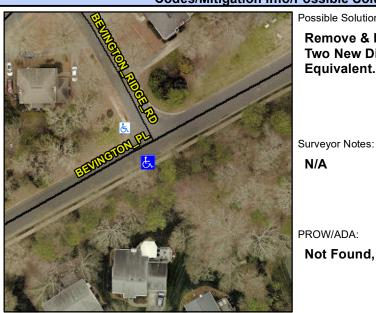
**BEVINGTON PL** Street 1 Name Stop Condition-Street 1 None Street 2 Name N/A Stop Condition-Street 2 N/A Possible Solutions: Remove & Replace Curb Ramp With **Two New Directional Ramps or** Equivalent.
