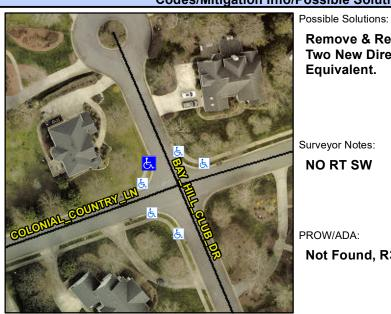
**BAY HILL CLUB DR** Street 1 Name Stop Condition-Street 1 StopSign Street 2 Name N/A Stop Condition-Street 2 N/A Remove & Replace Curb Ramp With **Two New Directional Ramps or** Equivalent.
