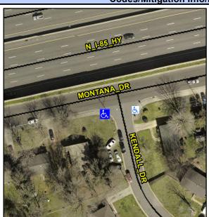
**KENDALL DR** Street 1 Name Stop Condition-Street 1 StopSign N/A Street 2 Name Stop Condition-Street 2 N/A Possible Solutions: Remove & Replace Curb Ramp With Two New Directional Ramps or Equivalent. Surveyor Notes: N/A
