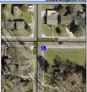
LASALLE ST Street 1 Name Stop Condition-Street 2 Street 2 Name Stop Condition-Street 1 StopSign Remove & Replace Curb Ramp With Two New Directional Ramps or Equivalent.
