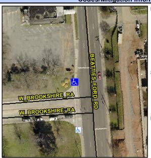
Street 1 Name Stop Condition-Street 2 Street 2 Name Stop Condition-Street 1 W BROOKSHIRE RA Signal **BEATTIES FORD RD** None Possible Solutions: Remove & Replace Curb Ramp With **Two New Directional Ramps or** Equivalent. Surveyor Notes: N/A PROW/ADA: Not Found, R304.2.2
