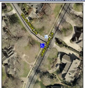
Street 1 Name Stop Condition-Street 2 Street 2 Name Stop Condition-Street 1 **JAMES JACK LN** None **VILLALONGA LN**  Possible Solutions: Remove & Replace Curb Ramp With Two New Directional Ramps or Equivalent. Surveyor Notes: N/A PROW/ADA:
