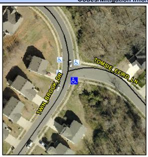
Street 1 Name Stop Condition-Street 2 Street 2 Name Stop Condition-Street 1 **TOMSIE EFIRD LN** StopSign **TWIN BROOK DR** None Possible Solutions: Remove & Replace Curb Ramp With Two New Directional Ramps or Equivalent. Surveyor Notes: N/A PROW/ADA: R304.2.2, R304.5.3
