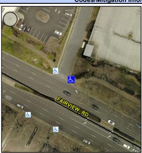
**ENTRANCE** Street 1 Name Stop Condition-Street 1 None Street 2 Name N/A Stop Condition-Street 2 N/A Remove & Replace Curb Ramp With **Two New Directional Ramps or** Equivalent.
